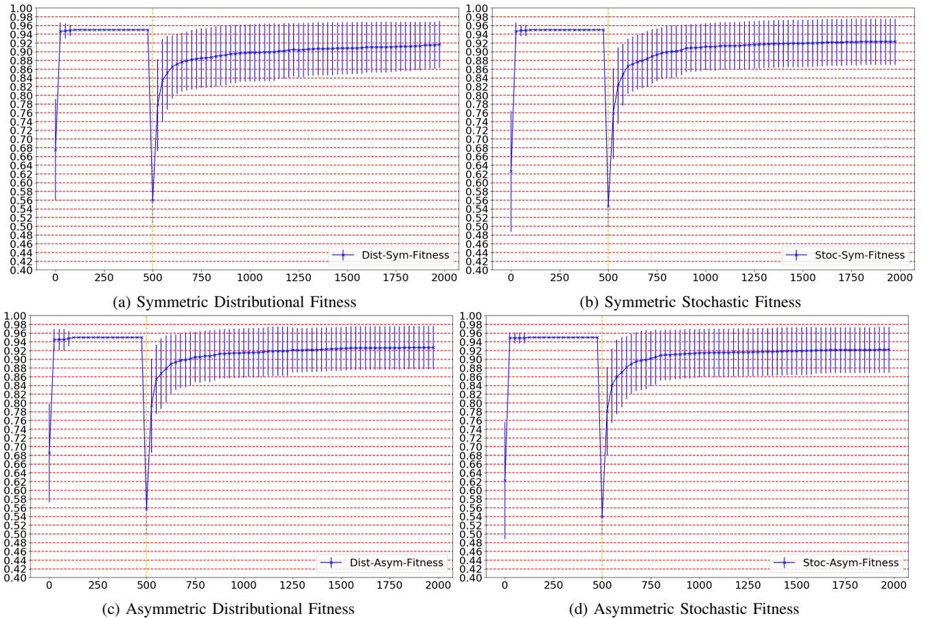
Fig. 9: Mean Best Fitness for each Generation over 100 Trials. Left to Right: Distributional vs Stochastic Evaluation. Top to Botom: Symmetric vs Asymmetric Fitness Function. Vertical bars represent one standard deviation. The vertical dashed line at generation 500 denotes addition of the second activation pattern.
